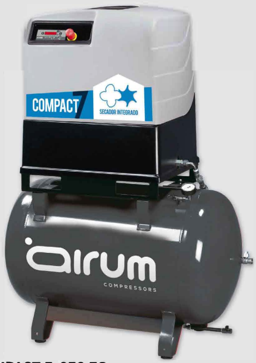
COMPACT 7-270 ES Airum 10 hp caldera 270 lts. 1000 lts./min. 400V III 10 bar. 67 dB(A).
